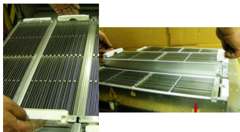
Fig. 46 Dismantling / Assembly of cathode sections
